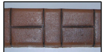
Spaced H-Brick (Black Grout)
